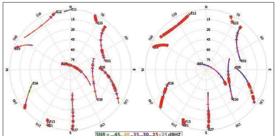
Figure 3. Skyplots showing the tracked Galileo satellites of the Google Pixel 5 on E1 (left) and E5a (right) with coloured visualisation of the Signal to Noise Ratio (SNR).
