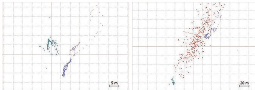
Figure 4. Comparison of PPP solutions for GPS (turquoise) and GLONASS (purple); on the left is point N09, on the right N07. Solutions for which only one SPP solution could be determined are shown in red. Note, the different scale of the grids.
