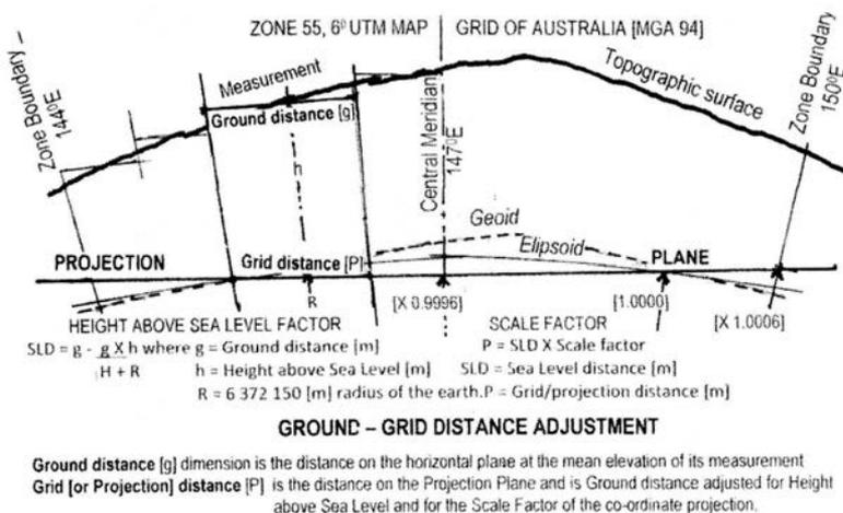
Figure 1: Ground distance to grid distance adjustment
